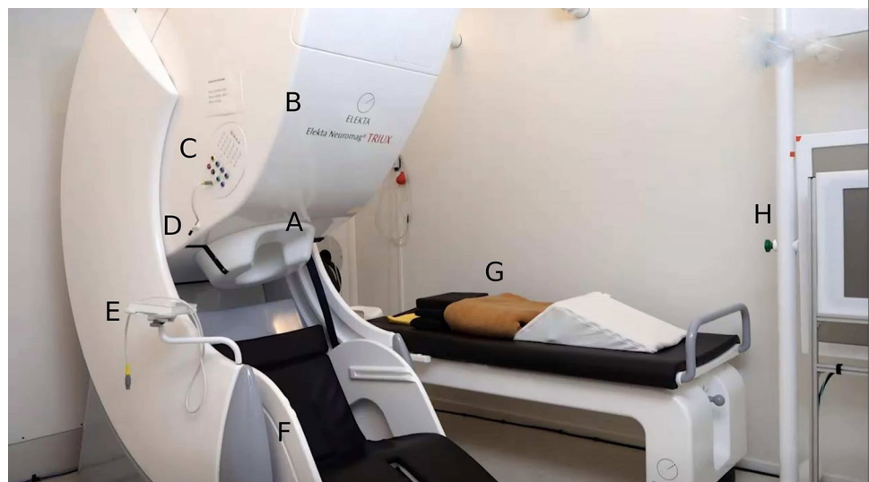
Fig. 2 Magnetoencephalography (device: whole-head MEG Triux, MEGIN Oy, Finland) within the magnetically shielded room (AK3b, Vacuumschmelze, Germany). A MEG-helmet with SQUID-sensor-unit. B Dewar with liquid helium inside. C EEG-unit with inputs for electrical signals (e.g., EOG, ECG). D Microphone. E Inputs for single EEG-electrodes. F MEG seat. G MEG bed. H Screen for visual stimulation
