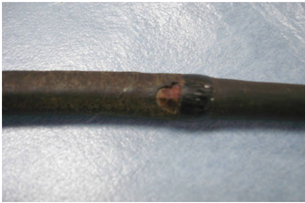
Fig. 2 Defect on the transesophageal echocardiogram probe. A biofilm was detected inside the damaged area. Specimens obtained by swabbing this area were positive for multidrug-resistant Pseudomonas aeruginosa (MDRP)
