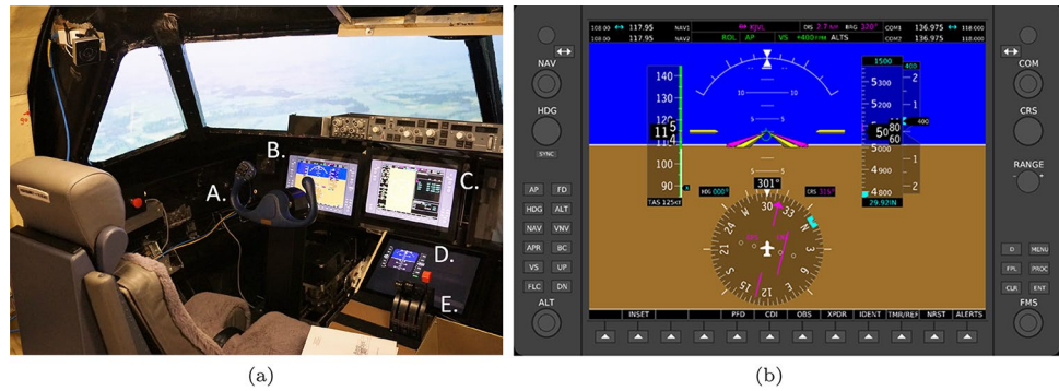
Fig. 1 a The experimental setup with: A. the control column, B. The Primary Flight Display, C. The Multi Function Display, D. The standby instrument, E. The throttle lever. b The Primary Flight Display used in the experiment
