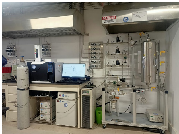
Fig. 7 Photo image from catalysis laboratory showing a 1-inch stainless steel fixed bed reactor and online gas chromatography used for gas conversion at Graphene Center of Excellence for electronic and energy applications, Egypt-Japan University of Science and Technology, Alexandria, Egypt
