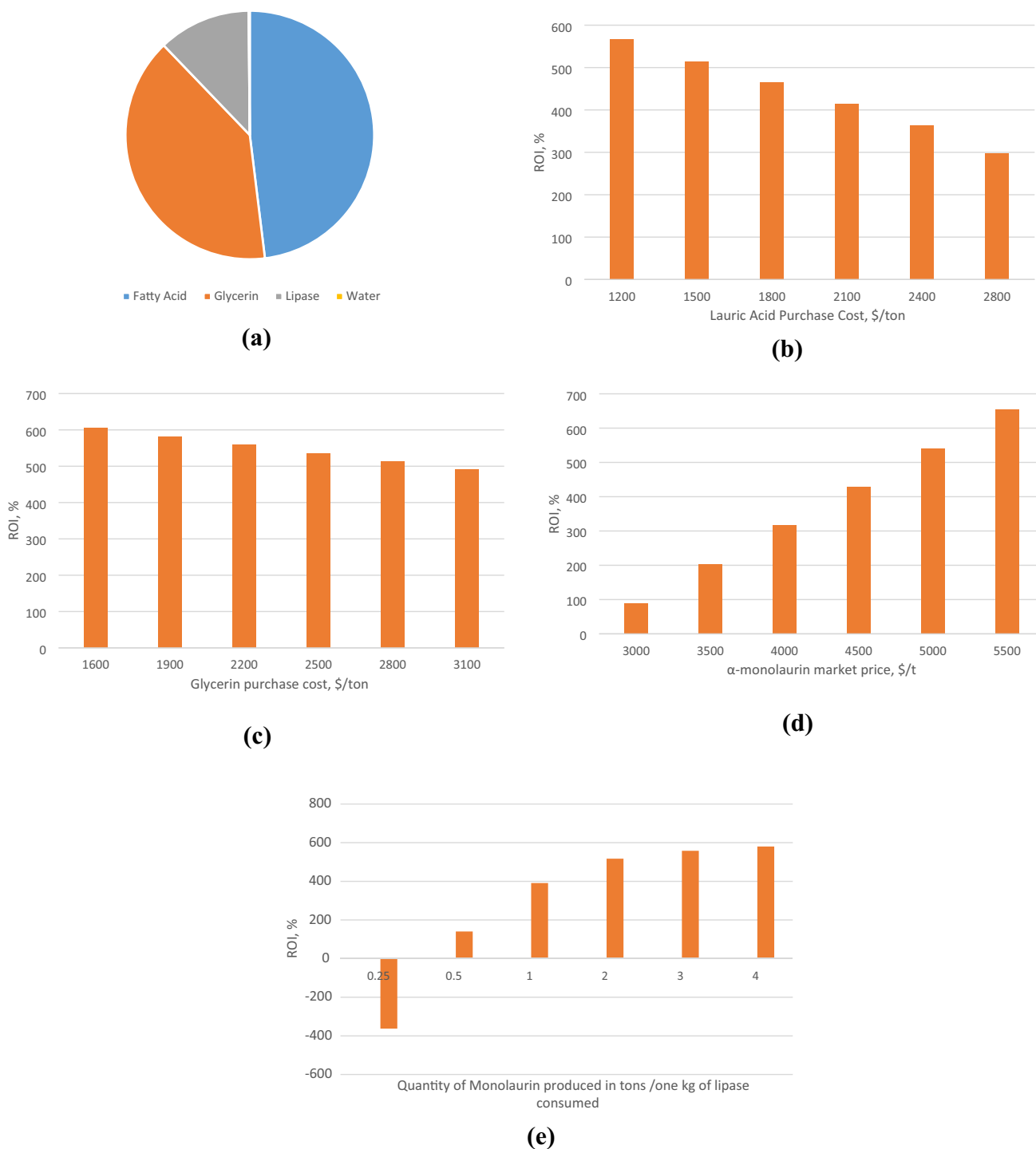
Fig. 3 Contribution of the individual raw materials used for monolaurin production. a Sensitivity of lauric acid purchasing price on ROI. b Sensitivity of Glycerin price variation on ROI. c ROI dependency on
