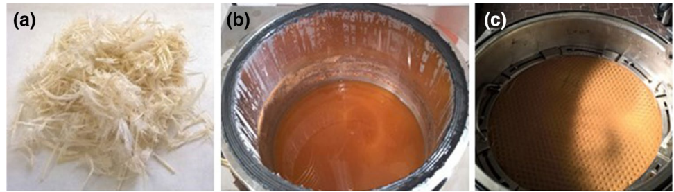
Fig. 3 a Waste chicken feathers, b hydrolysate, filtrate c filter cake
