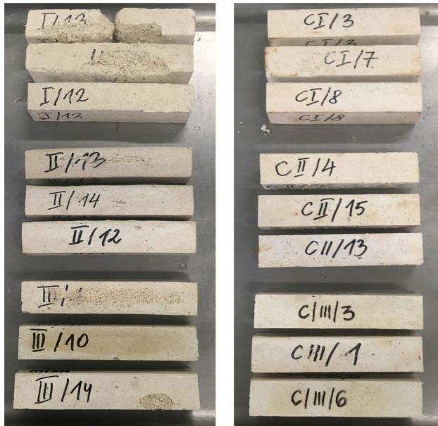
Fig. 6 Preservation conditions of PI/F, PII/F, PIII/F, CI/F, CII/F and CIII/F, samples after 25 freeze–thaw cycles and drying to the dry mass
