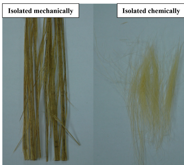
Fig. 3 Bamboo fiber bundles isolated mechanically and chemically, respectively
