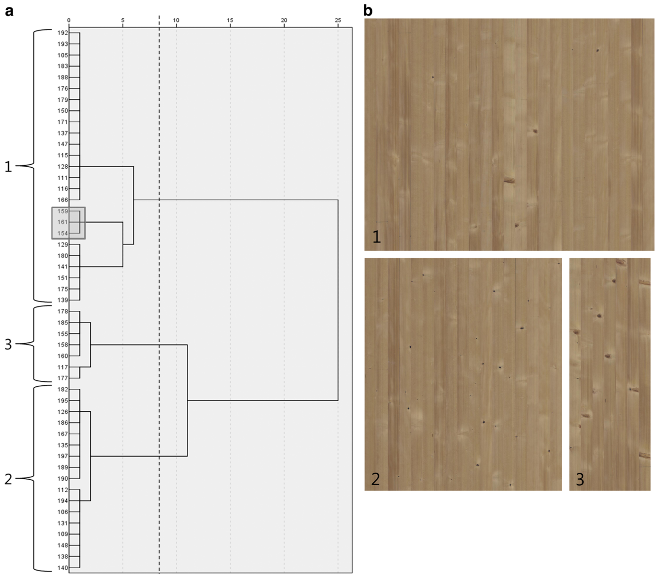
Fig. 12 a Dendrogram for the boards from the analysis sample in log-sector class 2 based on the variables included in the discriminant model. The horizontal scale indicates the distance coefficient, standardized to relative numbers in the interval 0–25, while the numbers on the vertical scale indicate the identifiers of the boards.
