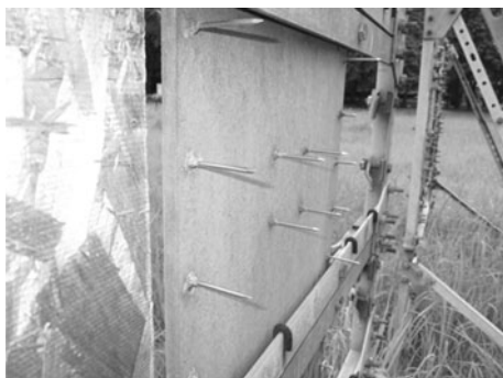
Fig. 1 Outdoor exposure test on boards with stainless steel nails driven in
