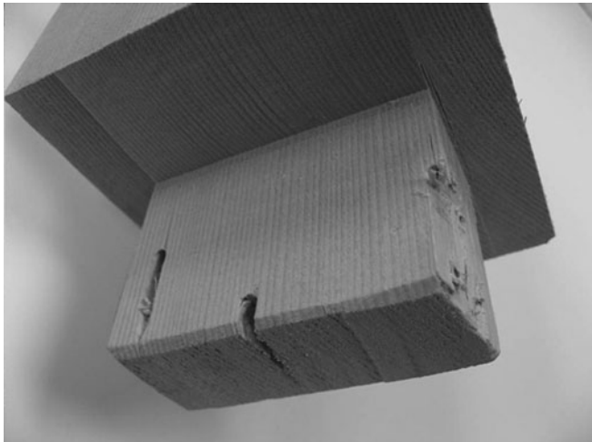
Fig. 9. Typical failure modes of the three nails penetrating the tenon: nail tear-out from tenon
