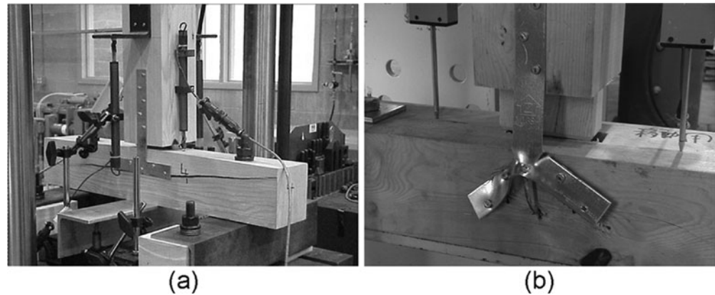
Fig. 7. Actual failure modes of the CPT connection under tension: a splitting on tension perpendicular to the grain, b nail pull-out and CPT plate in shear on a specimen with a short tenon 1,2
