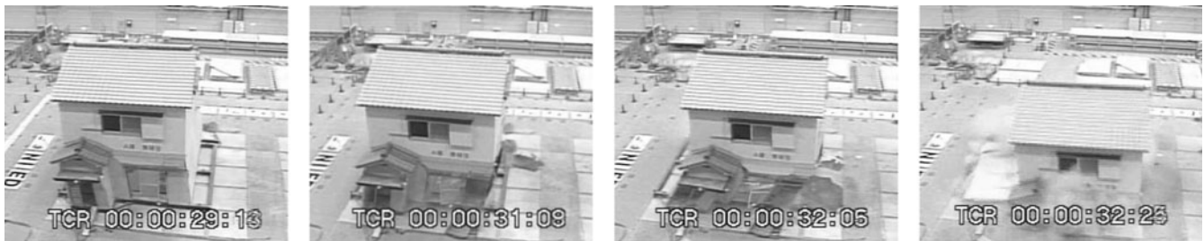
Fig. 14. Collapsing process of specimen in the shaking table test (JR Takatori)
