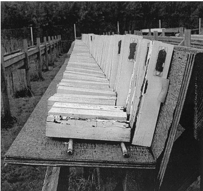
Fig. 1. The body of the L-joint tilted back 10° and the joint between the two specimens
