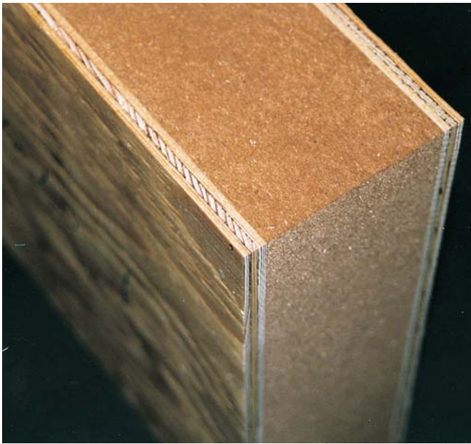
Fig. 1. Sample of the sandwich panel of plywood-overlaid low-density fiberboard (SW). Total board thickness is 96mm including a 78mm thick core and 9mm thick faces. The density of the specimen is 0.35\text{g/cm}^3
