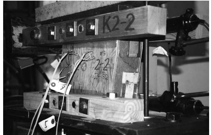
Fig. 12. Example of the ultimate stage of shear failure of SW. The direction of the surface grain of the face plywood is perpendicular to the loading direction. The density of the specimen is 0.41 g/cm 3 . Both face and core were crushed by the shearing stress. The fracture occurred around the neutral surface of the test specimen
