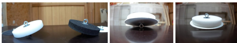
Fig. 3 Test stoppers: on top and inside the test box; training stoppers with integrated discs from different angles (below and above)
