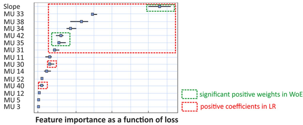
Fig. 6 Feature importance from the ANN model, including parameter slope and map units (MU) from BÜK200 and no sampling, with highlighted features considered also significant in WoE and LR models; with MU33: loamy-sandy molasse material, partly with a loamy flow-soil cover, MU38: clayey-loamy molasse material with a loamy top layer, MU34: silty to loamy molasse material, mainly with a flow-soil cover, MU42: loamy and sandy-loamy valley deposits, MU35: silty material of the freshwater brackish molasse, locally with loess-
