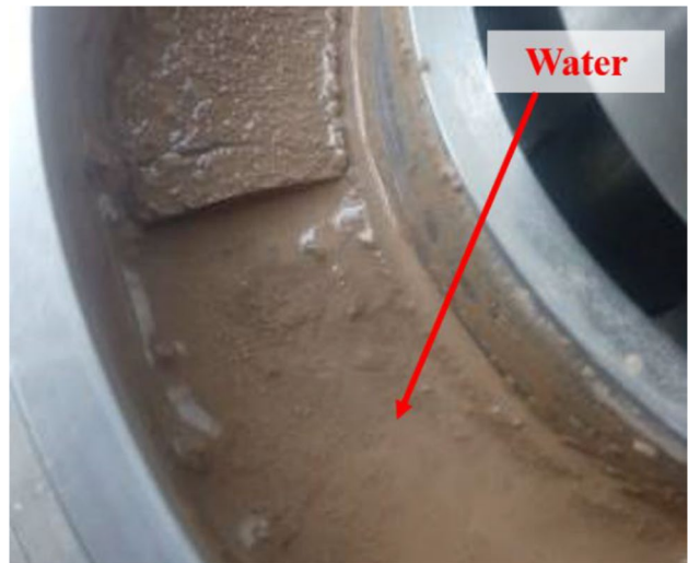
Fig. 12 Accumulation of water at the shear plane
