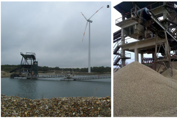
Fig. 2 Gravel pits operating with (a) bed dredging and (b) assorting system
