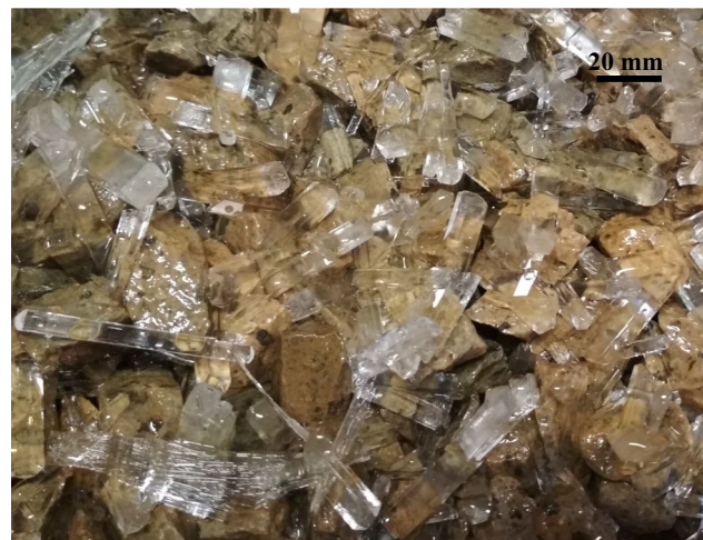
Fig. 4 Magnesium sulfate crystals on the grains of the aggregate sample of Andesite-2 (scale bar is on the right top)
