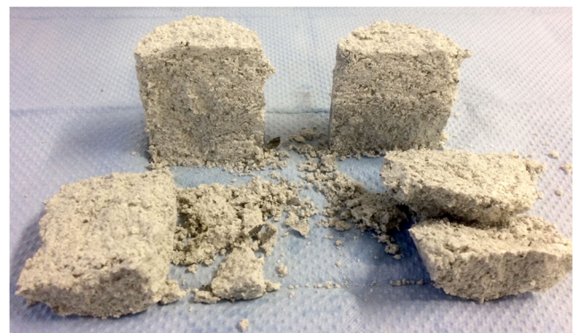
Fig. 11 Test sample 2-8 split after testing to check quality of water addition. In the case of dry zones, they were easy to detect
