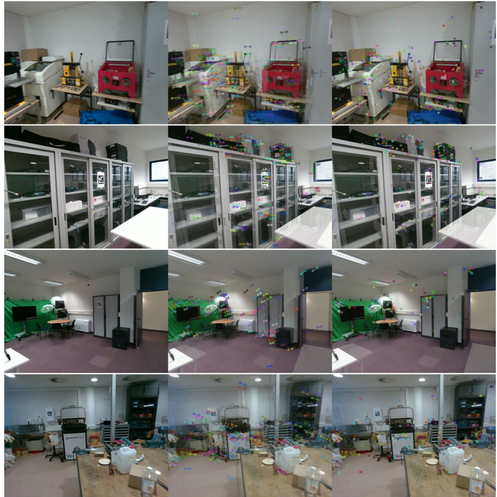
Fig. 5 Left: ground truth keyframe images as captured by the camera. Middle: overlay of the ground truth keyframe images with the rendered keyframe as estimated by SLAM. Misalignments are visible in the form of ghosting. The matched 2D features are visualized, which are used to quantify the displacement and to extract a ground truth keyframe pose. Right: similar overlay, but now rendered with the extracted ground truth keyframe pose, resulting in better alignment of the keyframe. Notice that the impact of moved objects between the acquisition of the 3D scan and the SLAM map keyframe is limited, as sufficient other features can be found. This is for example the case in the second example where the table has been moved
