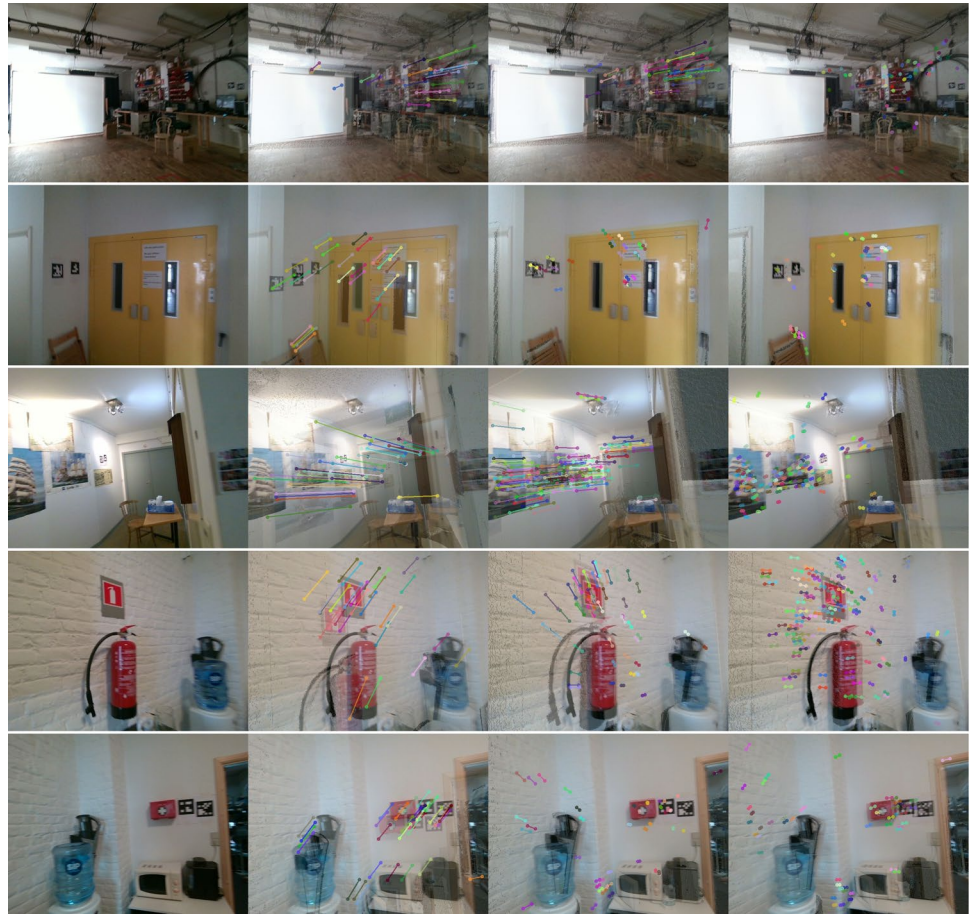
Fig. 11 Example results on a test sequence of the crew dataset. For the columns from left to right: (first) ground truth keyframe image; (second) overlay of the roughly aligned frame with the ground truth; (third) overlay of the marker-based aligned frame with the ground truth; (fourth) overlay of the keyframe-refined frame with the ground truth. For each blended pair, the figure shows feature matches and their respective distances
