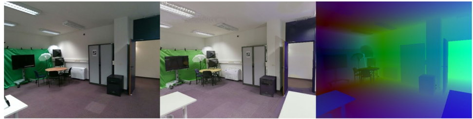
Fig. 4 Keyframe rendering. An example of a ground truth keyframe (left) and a rendered keyframe from the point of view of an estimated keyframe pose of SLAM (middle) and his accompanying 3D point cloud positions (right)
