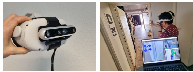
Fig. 6 Our XR camera setup with a Realsense D455 strapped to an Oculus Quest 2 HMD by a custom 3D-printed mounting bracket
