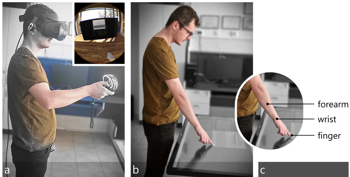
Fig. 1 a A user, wearing a head-mounted device, interacts with a virtual display in a virtual environment; b the same user interacting with a physical touchscreen display in the physical world; c locations on the interactive arm, progressively distant from the point of contact
