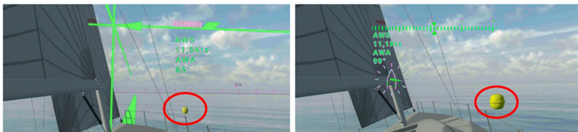
Fig. 1 The two visualization approaches tested: Boat (left) versus Head (right) stabilization
