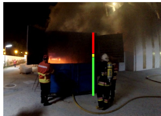
Fig. 4 Visual demonstration of the neutral plane phenomenon. The yellow bar demonstrates where the neutral plane phenomenon occurs, dividing the upper layer of superheated gases and smoke and the lower layer of oxygen
