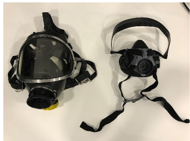
Fig. 2 Full face mask used in the RE (left) and half mask used in the VE (right)
