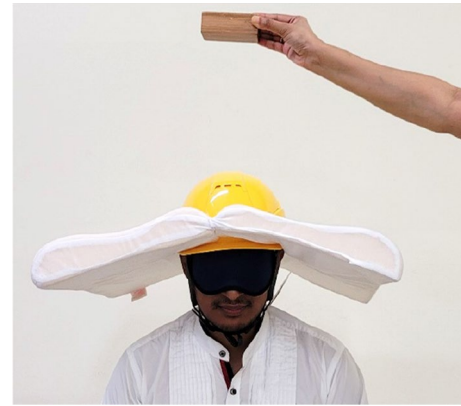
Fig. 12 Perceptual experiment. The participant compares the virtually rendered impact feedback and feedback from real objects falling. A safe guard was attached to the outside part of the helmet for safety reasons
