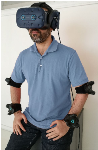
Fig. 2 The system's outfit consists of the VIVE Pro Eye VR HMD System and four vive trackers to monitor upper limbs movements
