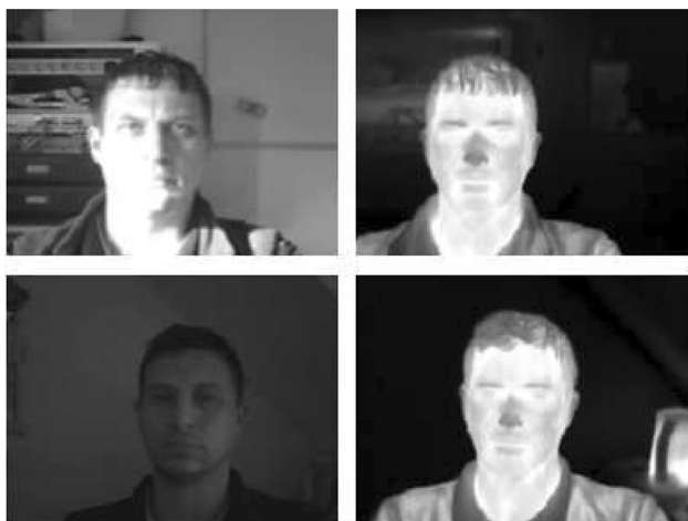
Fig. 1 Comparison of face images taken at the same moment in unfavourable lighting conditions using visible (left) and thermal (right) camera
