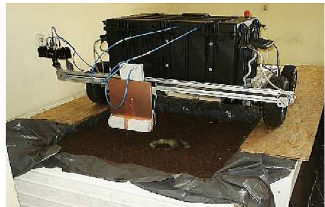
Fig. 3 Mobile GPR platform on in-door laboratory test stand
