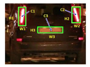
**Fig. 4** Detecting license plate and taillights. H, W, and C denote TLs and LP height, width, and center point, respectively, and numbers 1, 2, and 3 represent *left* TL, *right* TL, and LP, consecutively
