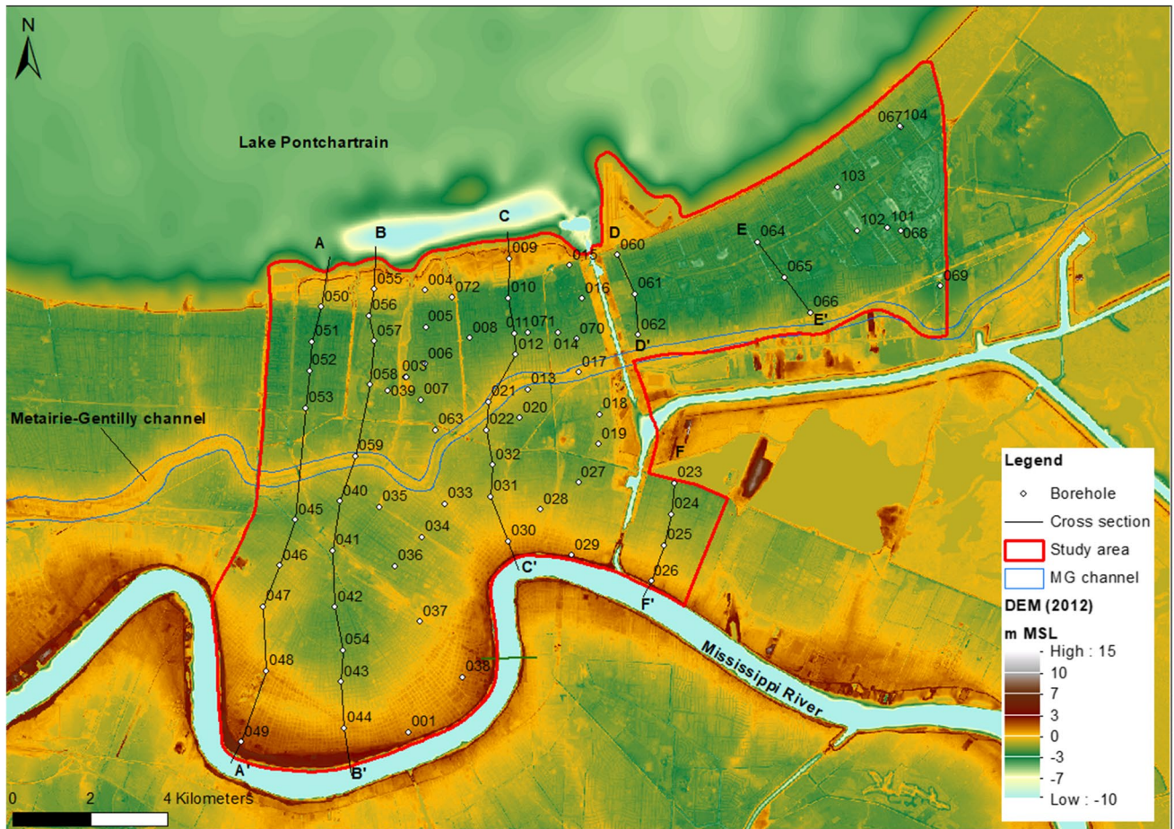
Fig. 6 Location of manually drilled boreholes and constructed cross sections. The approximate boundary of the abandoned Metairie-Gentilly channel is indicated by the blue lines. Source: digital elevation model (OCM Partners 2017)
