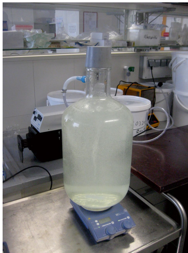
Fig. 2 Degassing of water via vacuum in a 50-L glass container using a water-jet pump (not shown) and a magnetic stirrer below the container, which aids in the expulsion of the gas bubbles
