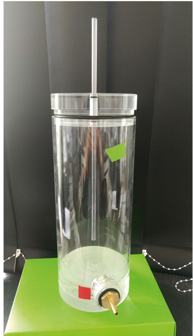
Fig. 5 Low-cost custom-made 2-L acrylic-glass Mariotte bottle with rubber seal at the top, ventilation pipe for maintaining constant pressure at different water levels, and a metal tube-connector outlet at the bottom. The height of this bottle is 35 cm
