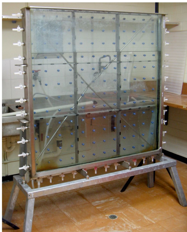
Fig. 6 Empty glass sand tank with steel framing and diagonal supports (sand tank dimensions are: 117.8 cm length, 120.0 cm height and 5.3 cm width). Equally spaced ports at the rear of the model are blue and in-/outlet connector valves at the sides and bottom to the (for example) Mariotte bottles are white (Werner et al. 2009)
