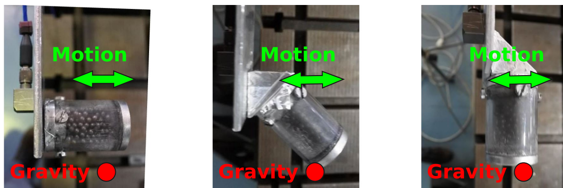
Fig. 3 Installation of the particle damper in the configuration orthogonal to the gravity. 0^\circ (left). 45^\circ (middle). 90^\circ (right)
