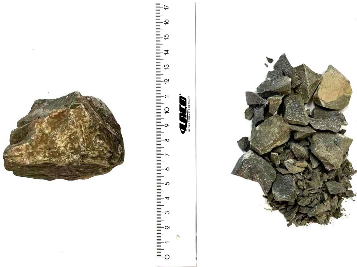
Fig. 1 Greywacke particle (equivalent diameter of 50 mm) from Breitenau (Saxony) before and after compression test
