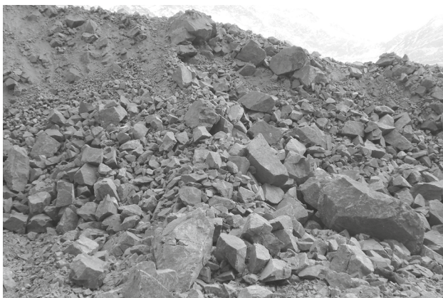
Fig. 2 Pile of blasted copper ore with an oversized boulder (Los Pelambres mine in Chile)
