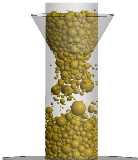
Fig. 6 Generation of the geometrical model a filling the container with loose particles
