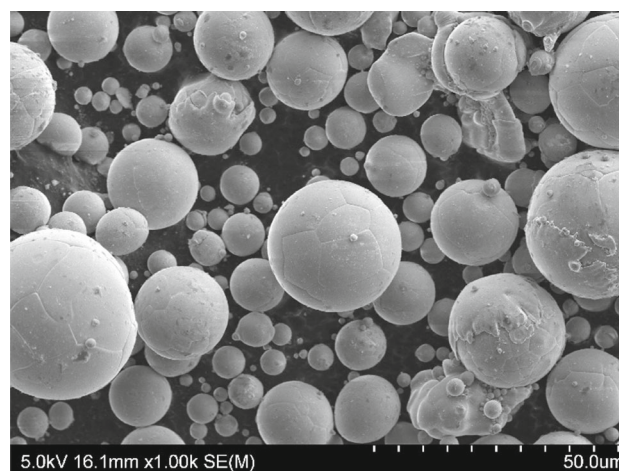
Fig. 7 Morphology of the NiAl powder after compaction process up to 50 MPa
