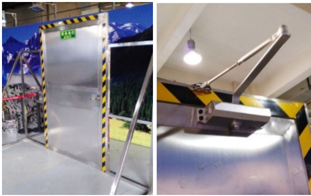
Figure 10 Door and door closer in the experiments
