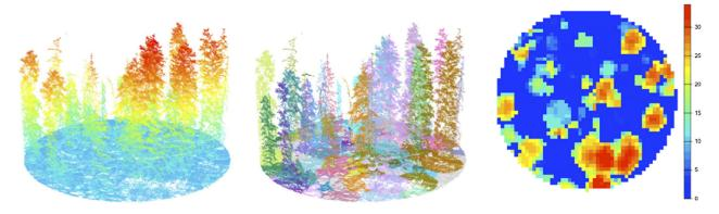
Figure 2. Examples of a LiDAR point cloud for a  $500 \text{ m}^2$  forest research plot (left plot) with individual trees segmented to derive tree based structural metrics (for example, height; middle plot). The data were collected from a helicopter in 2021 and processed using the open-source lidR package (Roussel and others 2020). The right plot shows a canopy height model derived from the point cloud at a spatial grain of  $1 \text{ m}^2$ .
