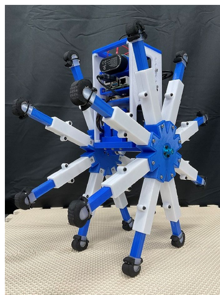
Fig. 12 Rimless wheel robot with elastic telescopic-legs
