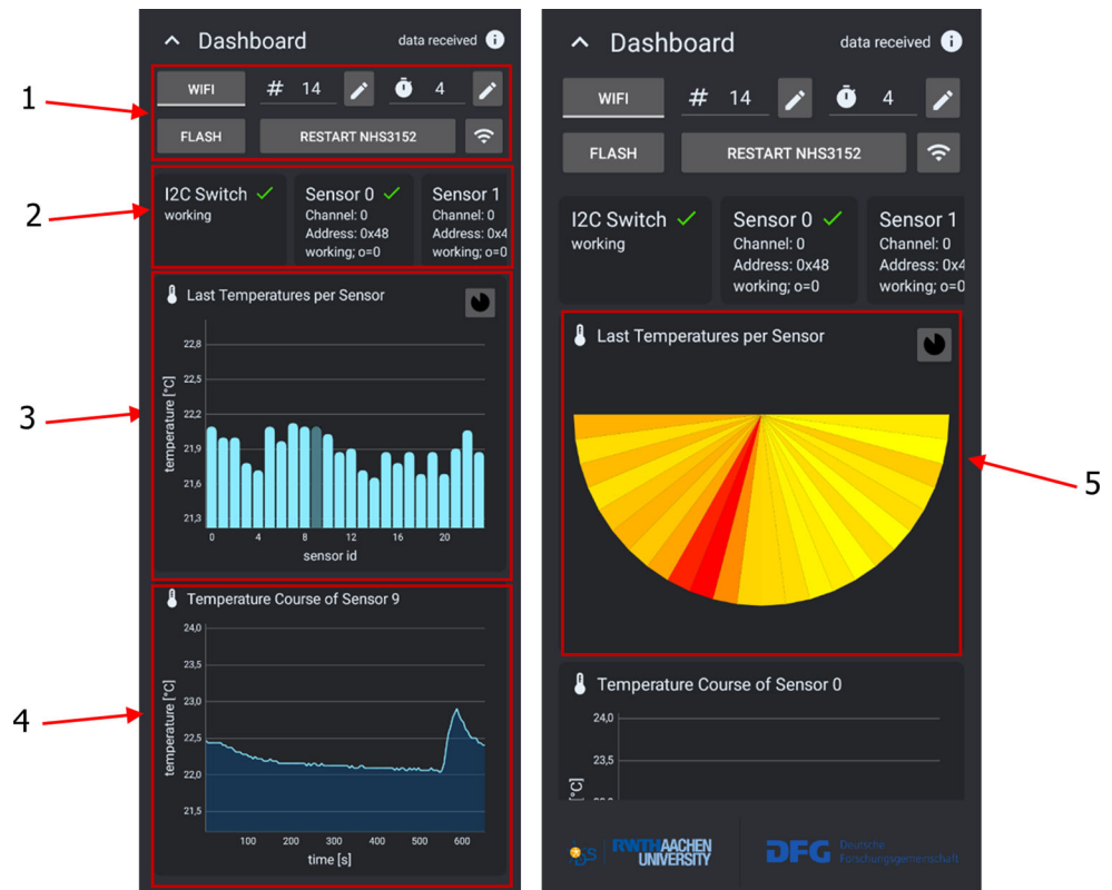
Fig. 9 Dashboard of the Android application for monitoring the plain bearing. (1 Control panel to change temperature precision, edit the deep sleep duration of the microcontroller, flash the NHS3152 wirelessly, restart the sensor system or switch between the hosted WiFi network and an existing WiFi network, 2 Status overview of the components, 3 Temperature overview of all sensors, 4 Temperature course of the selected sensor, 5 Different view on the data of 3 [view can be alternated by clicking the button in the upper right corner])
