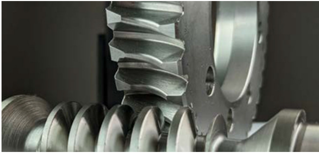
Fig. 1 Cast iron worm wheel (with corresponding worm in the foreground)
