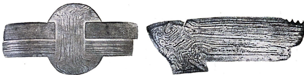
Fig. 6 Imprints of the surface of two iron specimens obtained by A.I. Glazunov using electrography [35]
