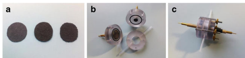
Fig. 1 (a) Carbon paper, carbon fibre and carbon cloth electrode substrates before modification with MWCNTs. (b) Cathode, anode contact and reaction compartment of the cell. (c) Fuel cell assembly working under flow conditions
