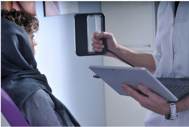
Fig. 1 The scanning process of the face in a patient with the Sense 2 scanner
