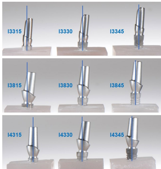
Fig. 5 Exemplary deflections of all test groups after load-to-fracture test
