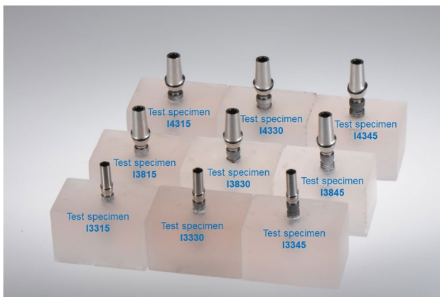
Fig. 3 Test specimens with their diameters (3.3, 3.8, and 4.3 mm) and simulated bone loss (1.5, 3.0, and 4.5 mm) representing all 9 groups
