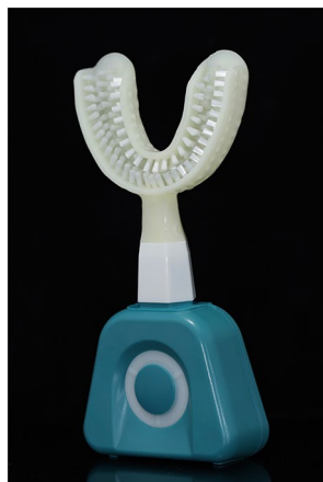
Fig. 1 The auto-cleaning device Y-brush ®. The single-sided and flexible mouthpiece is mounted with six rows of nylon bristles at the occlusal, oral, and vestibular side of the jaw. Bristles are aligned in 45° against the tooth surfaces to simulate the bass method. It must be rotated to the left and right during the cleaning process additional to gently and quickly chewing on it [15]
