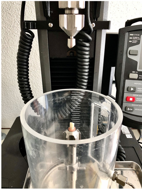
Fig. 3 Specimen positioning with the cemented primary crown in the test device before luting of the secondary crown in the tertiary structure, which was positioned in the upper collet
