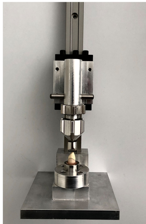
Fig. 1 Customized device for standardized base plate fabrication for the artificial tooth and cementing of the primary crown
