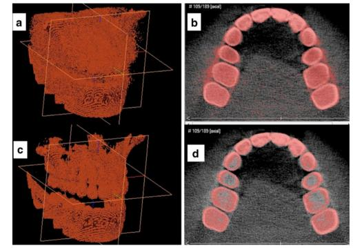
**Fig. 1** An example of the segmentation procedure and threshold value determination for a 3D model from group (C) in 3D (**a**, **c**) and on 2D axial slices (**b**, **d**). The model can have an increased noise level due to threshold underestimation (**a** and **b**) or several holes in the bone and teeth due to threshold overestimation (**c** and **d**)
