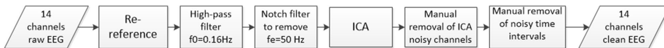
Fig. 2 Pre-processing on the raw EEG data for each of the fourteen channels
