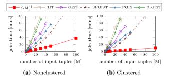
Fig. 15 Overlap join with equality predicates for synthetic data by varying the cardinality of both relations
