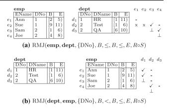
**Fig. 3** Range–merge joins for our running example:  $\checkmark$  indicates a match,  $\perp$  the end of matches, - an inner skip, and x an outer skip
