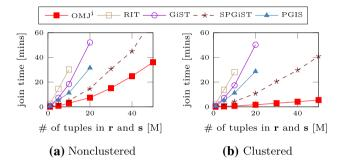
Fig. 12 Overlap join without equality predicates on synthetic dataset, varying number of tuples of both relations
