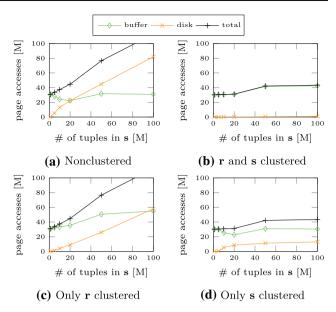
Fig. 22 Page access for the first range join of the overlap join
