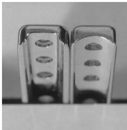
Fig. 10. Railed plates ( left ) have limited bone–plate contact area compared to contact plates ( right )
