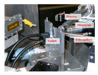
Fig. 3 The experimental table showing the sample holder arrangement at beamline L at HASYLAB
